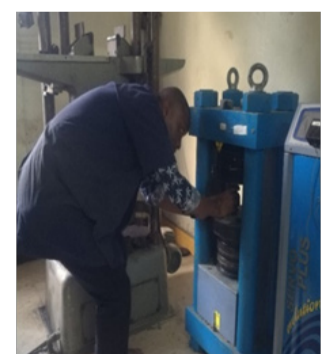
Figure 3: Rock strength test data acquisition in a Uniaxial Compressive Strength (UCS) machine.
