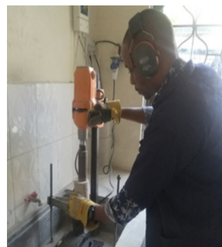
Figure 1: Rock core sample preparation (resizing) for Uniaxial compressive strength test.
