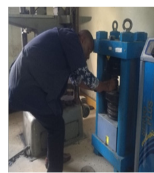
Figure 2: Rock core sample placing between plates of Uniaxial compressive strength machine for the test.
