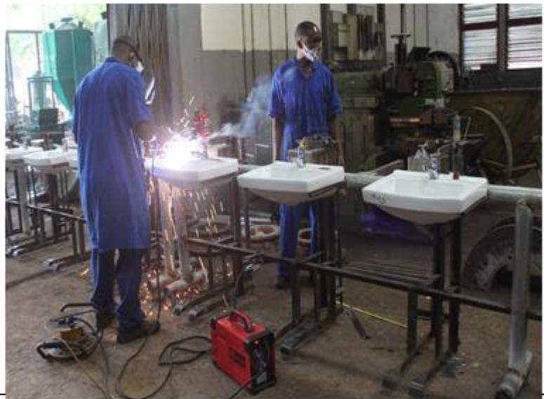
*UDSM Engineers fabricating special hand washing machine*
